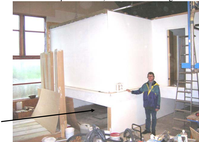
Figure 9 Photograph of the laboratory apartment, the arrow points into the crawl space beneath the ceiling.
